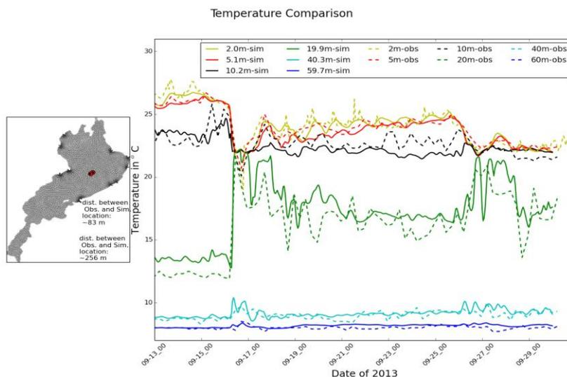
**Figure 1:** Left-hand side: grid used in the simulation with the locations of the monitoring stations (red circles) and closest points in the simulation (black circles). The distance between the locations is written. Right-hand side: comparison of simulated temperature time series (solid lines) against observed temperature time series (dash lines)
